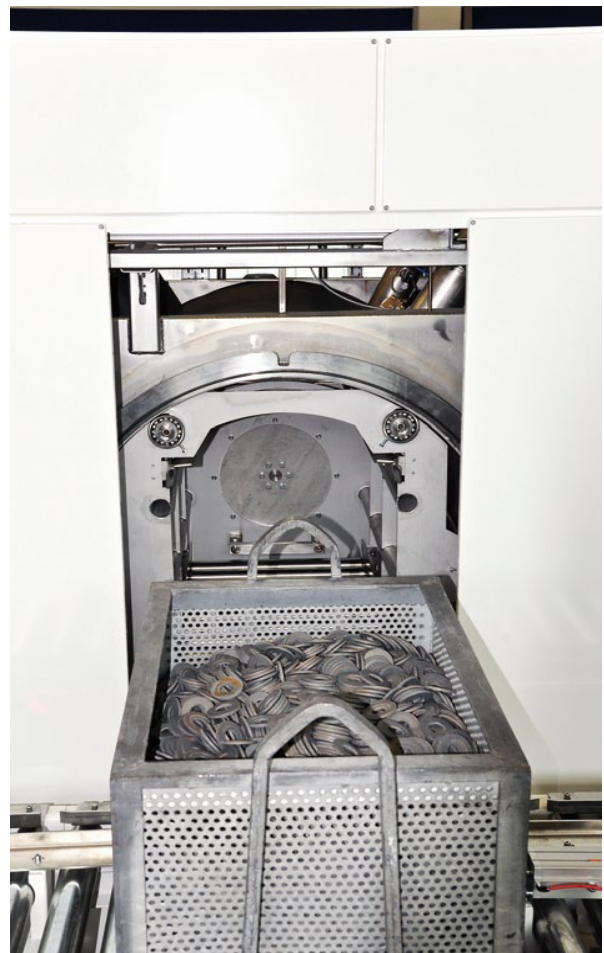
The parts are cleaned in 850 x 600 x 750 millimetre baskets as tightly packed loose material
