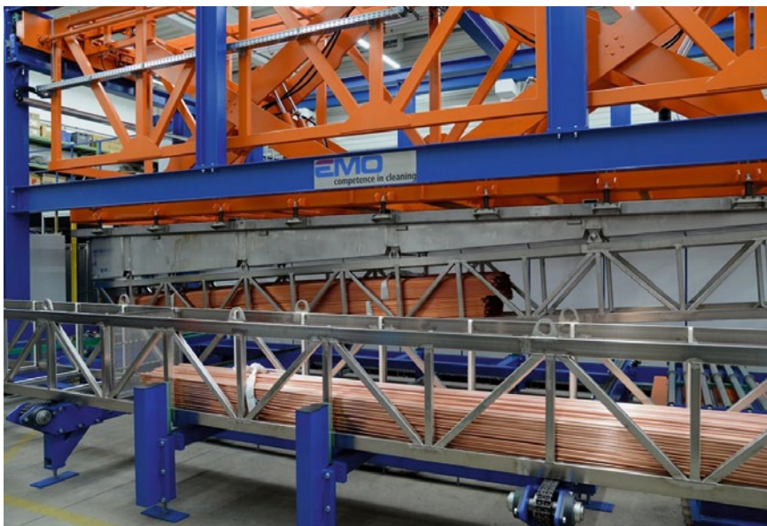
While the front parts container waits to be unloaded, the batch at the back is making its way into the cleaning chamber.
