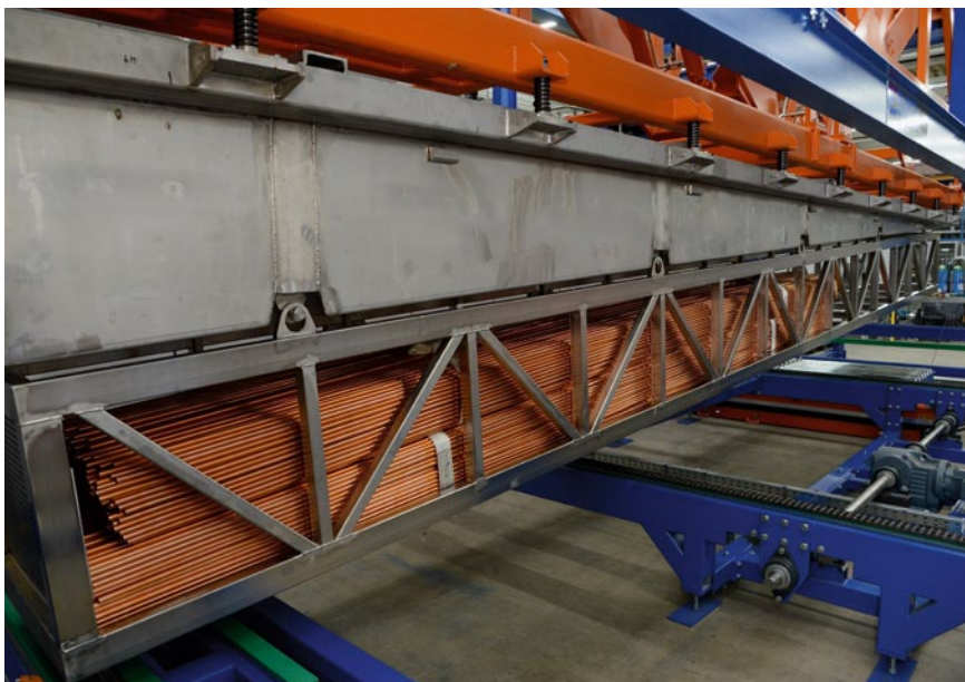
The angle of the container helps the cleaning process and allows the chamber to be emptied quickly.
